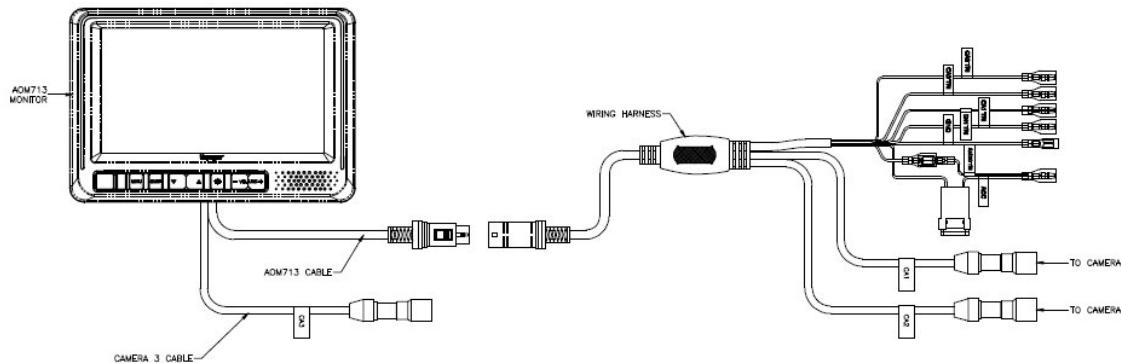
If you need more length for your application, you will need to extend your power/trigger wires and pull additional camera cable up to the monitor's harness or use an additional camera cable to extend the existing cable (p/n **CEC15** -15 ft.).
