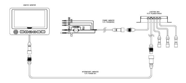
Install the **AOM713** monitor panel and wiring harness in place of the old system. Your camera cable will connect into the **TO CAMERA** inputs.
